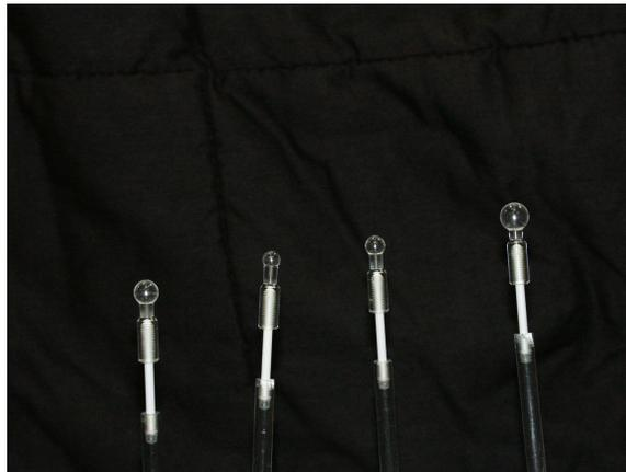
Figure 4.3. Photo of the micro-hollow spheres used to simulate lesions.
