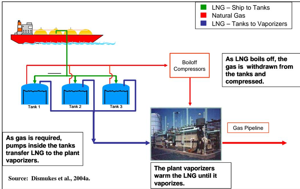
**Figure 36. Receiving Terminal – LNG Gas Flow.**
