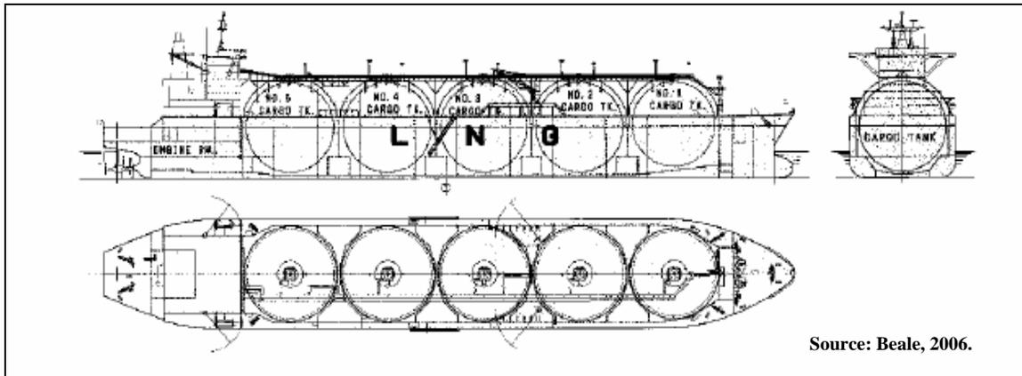
**Figure 57. LNG Tanker Design with Spherical Tanks.**
