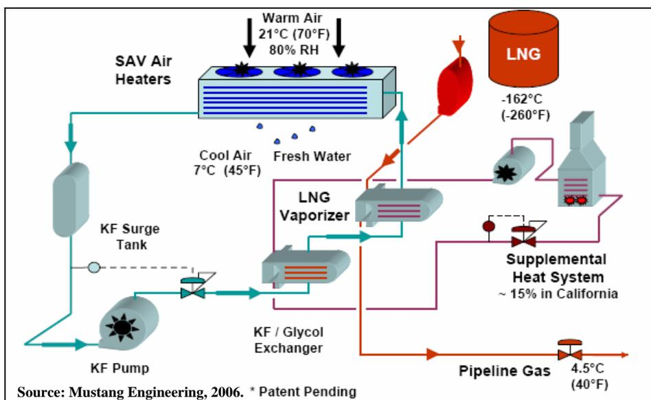
**Figure 70. Mustang LNG Smart™ Ambient Air Vaporization Process.**
