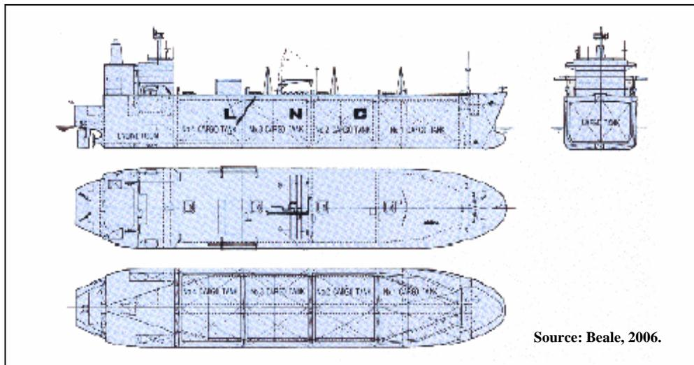
**Figure 60. LNG Tanker Design with Prismatic Tanks.**
