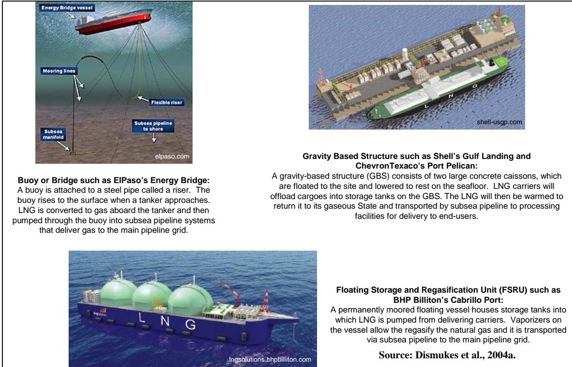
**Figure 38. Types of Offshore LNG Receiving Terminals.**
