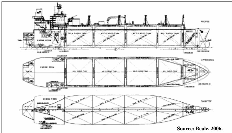
**Figure 62. LNG Tanker Design with Double Membrane Tanks.**
