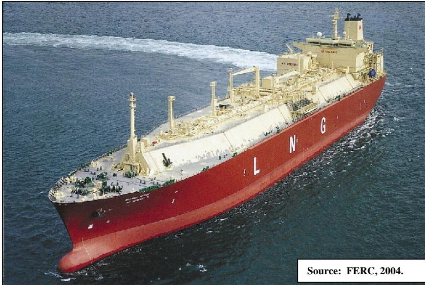
**Figure 59. LNG Tanker with Prismatic Tanks.**
