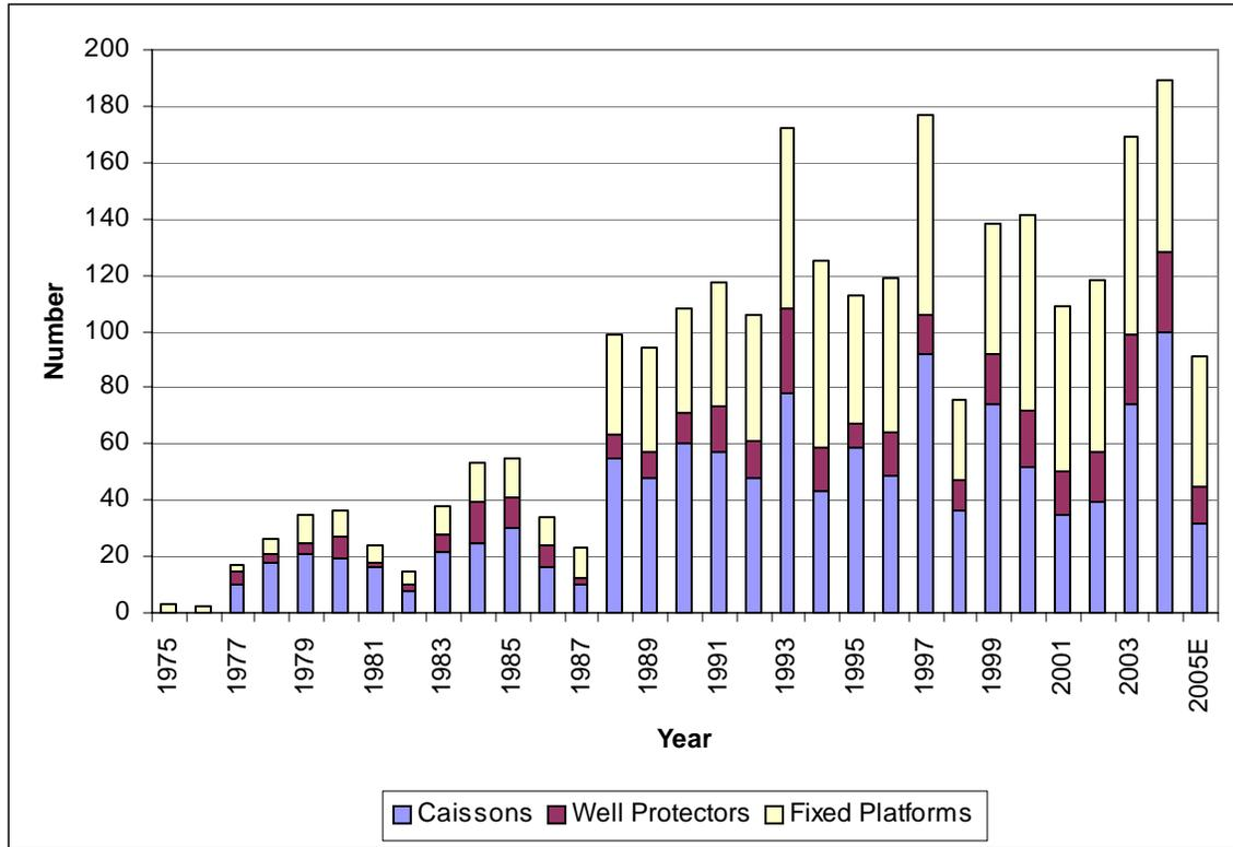
**Figure A.1. Structures Removed in the Outer Continental Shelf of the Gulf of Mexico, 1973-2005 (Data for 2005 as Reported on March 3, 2006 and Indicated as 2005E).**
